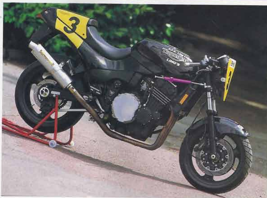
This is what you get with just a pipe, 155 main jet and a simple air box modification : 95bhp as opposed to 90bhp standard and a smooth, creamy power curve without the old lumps
