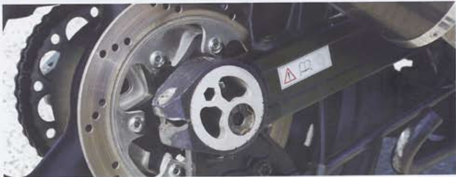
Rear anchorage is provided by a disc, and chain adjustment is achieved by rotating the eccentric spindle carrier, a system familiar to contemporary Kawasaki owners
