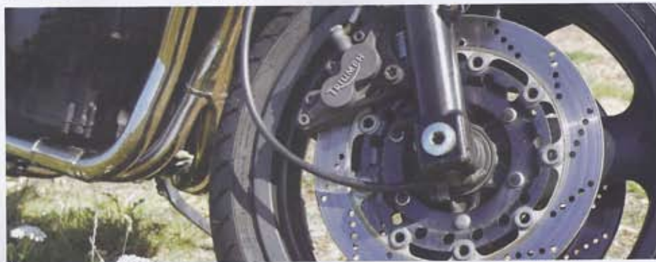
The Speed Triple's front end is conventional for its day, no tricky suspension systems to worry about. Anchorage is effective; a pair of floating rotors gripped by 4-pot callipers pull the speed down smoothly
