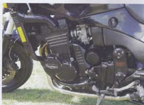
The driveside view of the engine suggests that it was never intended to be on view! There are feeble attempts to 'style' away the plumbing, for example. The fuel tap is the most sensible in the world and the oil filler stands out like a large hint...
