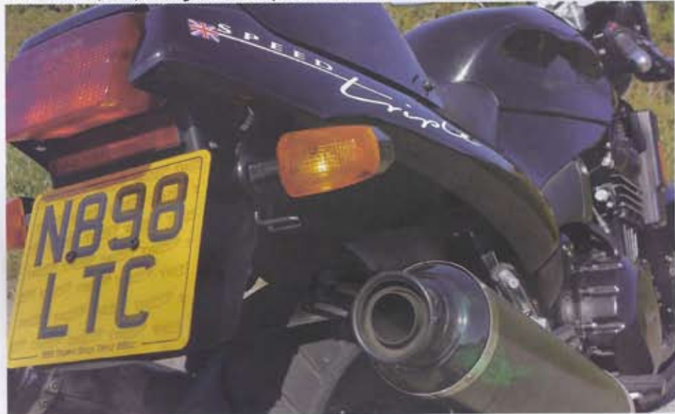
The 'carbon fibre' exhaust cans are in fact steel cans with wrap-around sleeves
