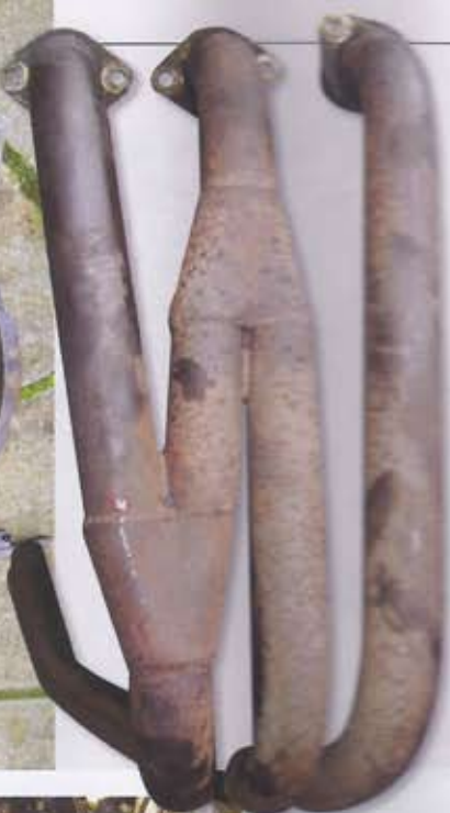
Exhaust before being vapour blasted
