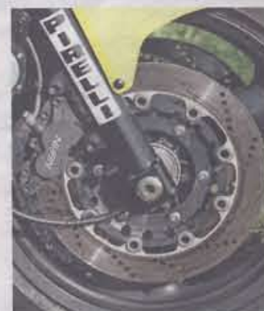
Forks were beefed-up by Maxton, but brakes use standard road-bike parts
